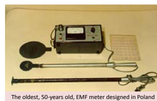
The oldest, 50-years old, EMF meter designed in Poland
